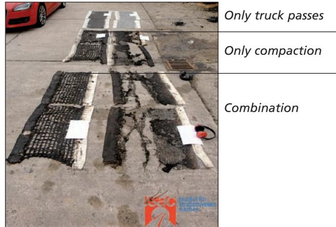
Figure 7.: Results of installation damage test
